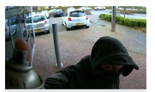
Tamper Detection An alarm is triggered automatically when the camra detects someone attempting to cover, vandalise or move the lens.
