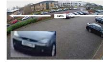
ZMR6522 Lens set to 3.3mm Distance to target: 30m
